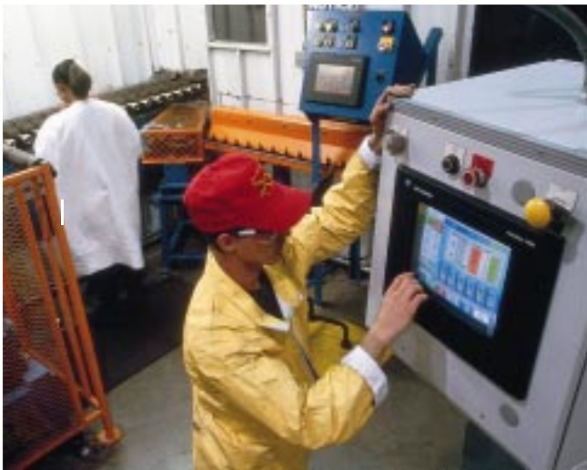
Kwikset uses RSSql for bi-directional communication via Ethernet between engines and a SQL database.
